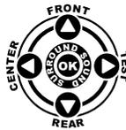
In the **AUDIO** mode, use the **Cursor Keys** to move the cursor to select or test surround sound channels on your audio device. Also see **VOL** keys (above left).
